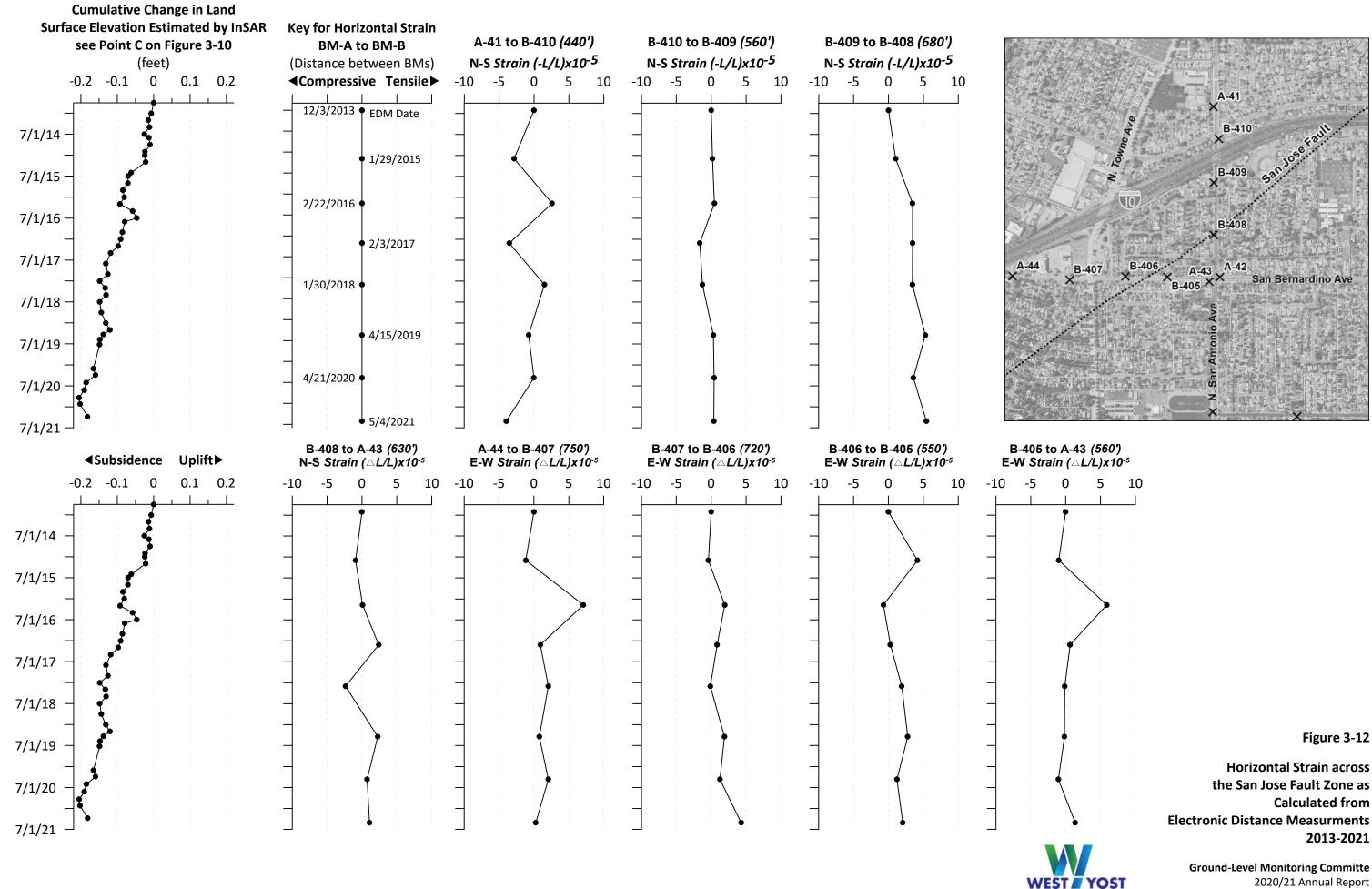
**Horizontal Strain across** the San Jose Fault Zone as **Calculated from Electronic Distance Measurments** 2013-2021
