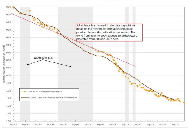
The Model-Simulated deformation vs InSAR-Estimated ground motion figure is reproduced Model-Simulated Aquifer-System Deformation versus InSAR-Estimated Ground Motion at the Pomona Extensometer Facility for the Final Calibrated 1D Model
